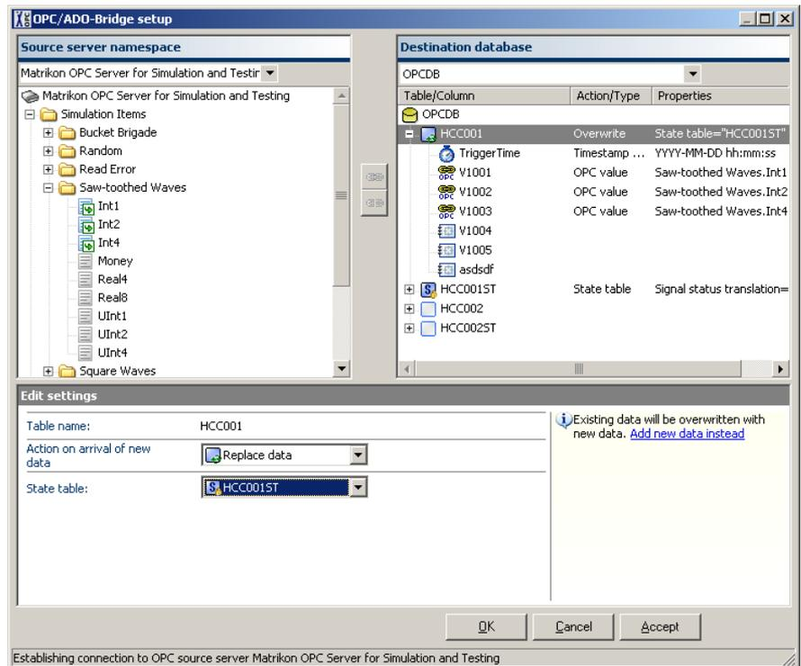
After confirming all changes and closing the dialog the bridge is setup completely and the data transmission can start. The main window should now show some information about the OPC source server, the ADO destination database and the transmitted data.
