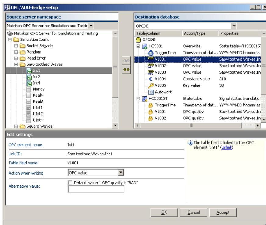
The setup dialog is split up into three regions. In the upper left area the OPC source server and its namespace is shown. To the right the structure of the selected database is shown. More information for the currently selected items are shown at the bottom of the dialog.
