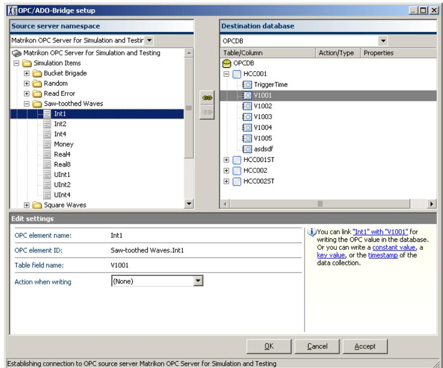
This procedure needs to be repeated for each OPC item that should be stored in the database. Apart of the OPC data also the timestamp of the transmission can be stored by selecting the respective column in the database and changing the **Action when writing** to **Timestamp of data collection**.
