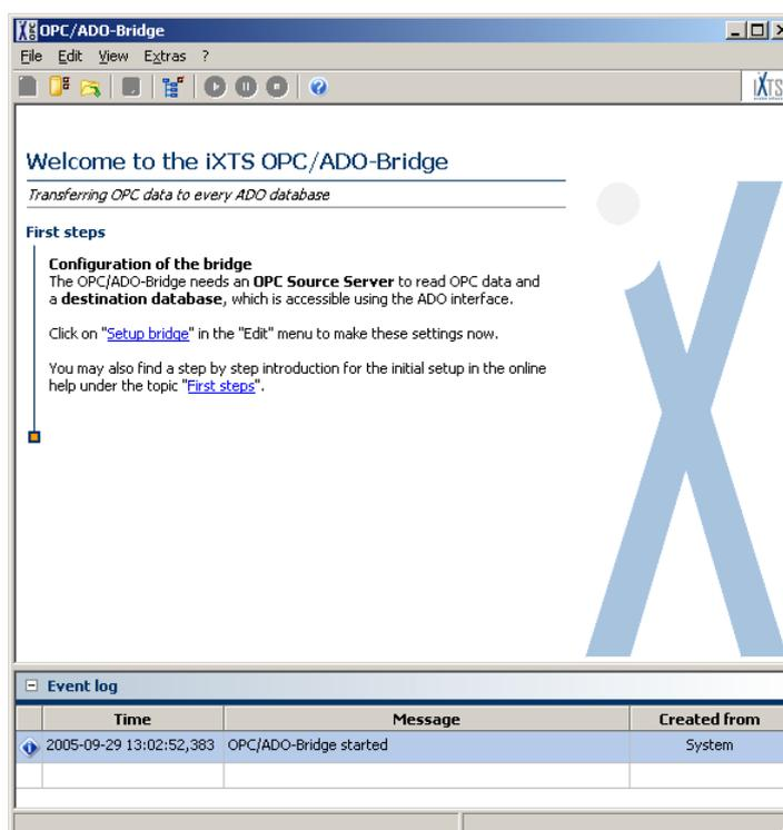
To start working with the bridge an OPC Source Server and an ADO destination database need to be defined and the OPC elements which should be stored in the database must be selected.
